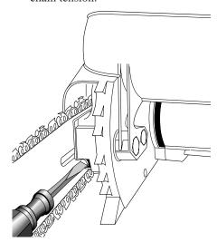
Figure 5 - Turning Adjusting Screw
